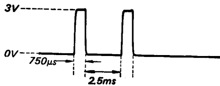
(BE) 0V DC WHEN AM SWITCH IS PRESSED TWICE OR a1 THROUGH d8 SWITCH IS PRESSED ONCE, MOMENTARILY ONE PULSE.
