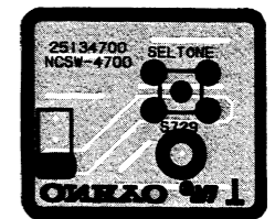
STC SWITCH PC BOARD
