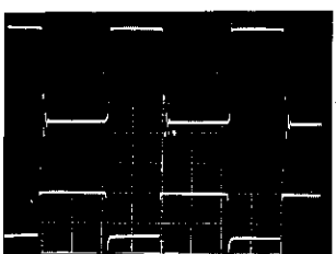
(Upper) T901 pin (6) (CAM 16.5V) (Lower) Q940 Collector 10V, 1µsec/div
